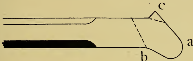
Fig. 97. Correct shape of punch bar.
